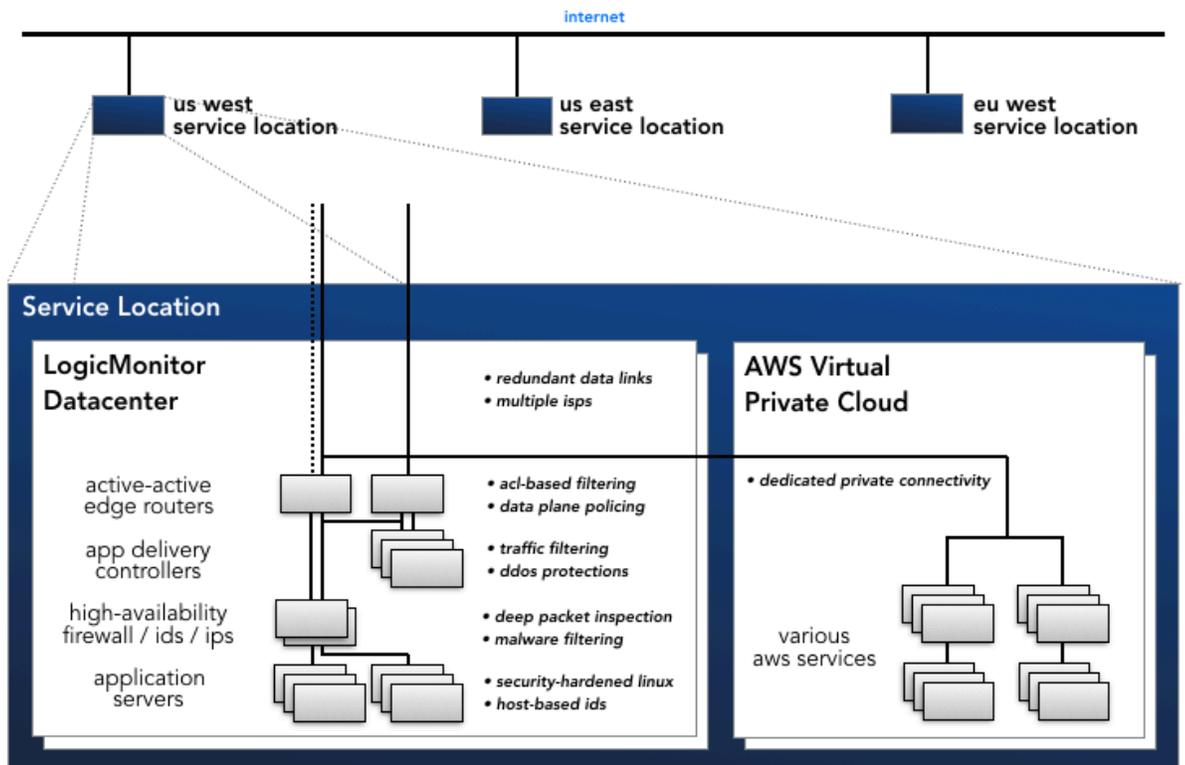
Figure 2. LogicMonitor Platform – Network & Security Topology
