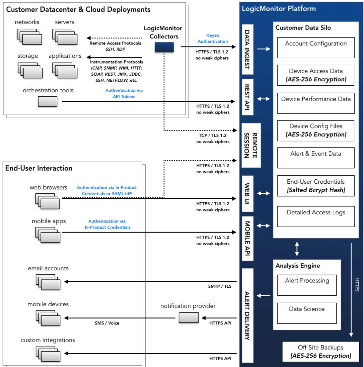
Figure 1. LogicMonitor Platform – Data Flow Overview
